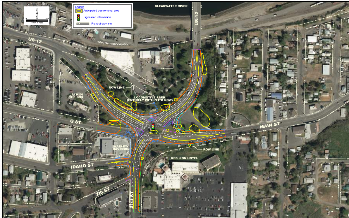
Figure 5. Areas of Vegetation Removal
