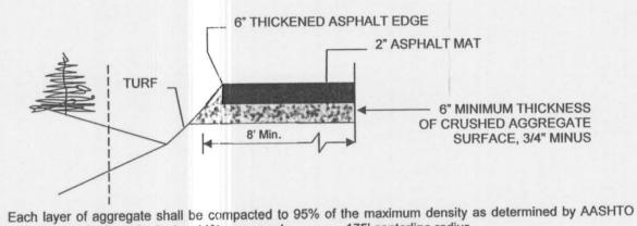
T99-70, standard proctor test. 11% max. grade 175' centerline radius 15-20' corner radius Swale drainage This standard shall apply to all new accessways on private property that serve dwellings and storage
