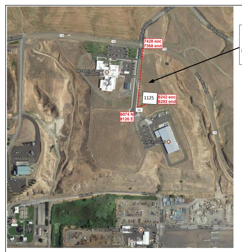
PULL ONE 48CT. SINGLE MODE ARMORED FIBER OPTIC CABLE 800' THROUGH EXISTING 2" CONDUIT. LEAVE 50' SLACK IN EACH HH.
