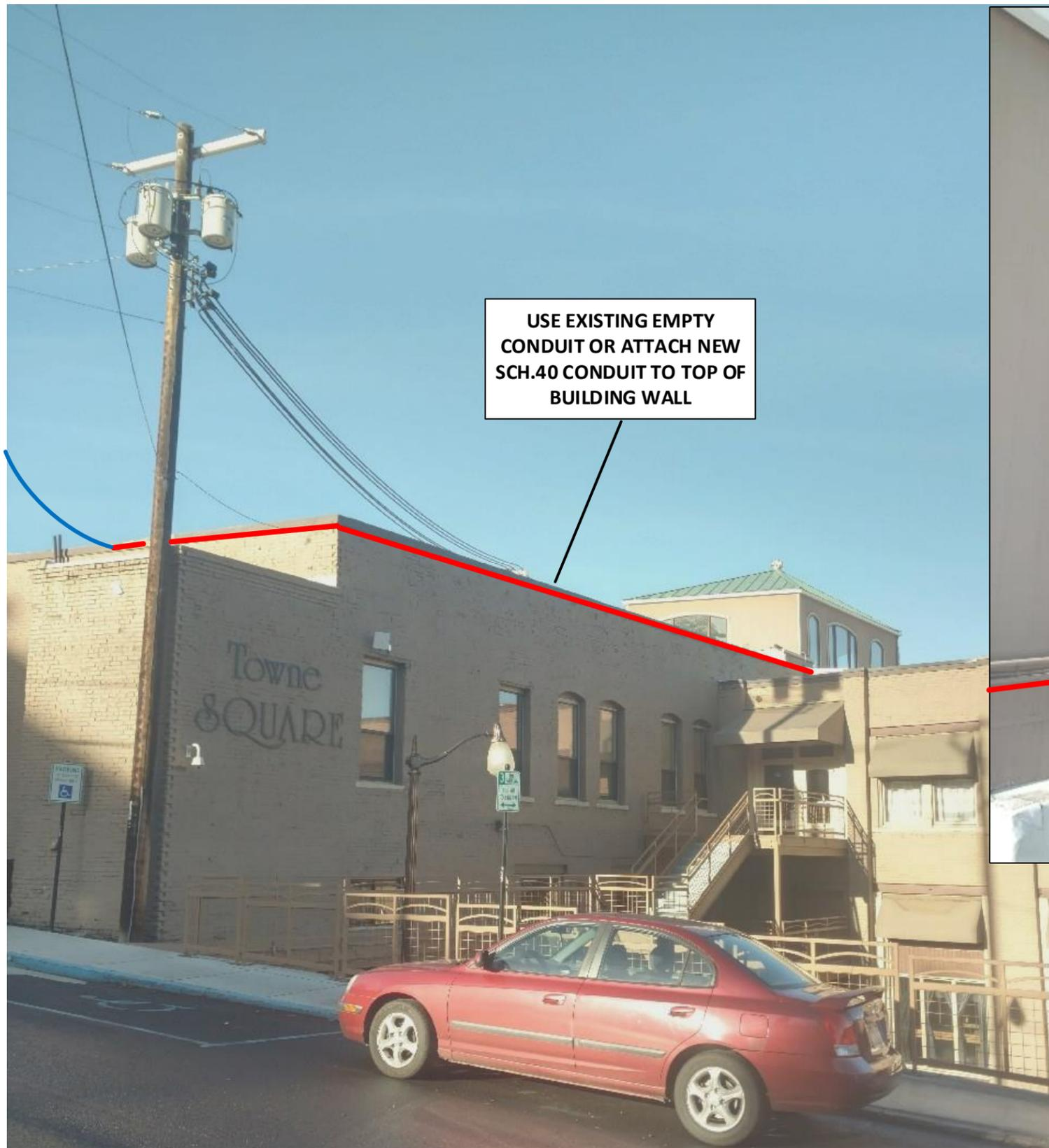
USE EXISTING EMPTY CONDUIT OR ATTACH NEW SCH.40 CONDUIT TO TOP OF BUILDING WALL
