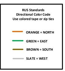
ALL BFO'S WILL HAVE DIRECTIONAL COLOR CODE MARKER LOCATED 24" FROM CONDUIT ENDS AND 24" FROM END OF BFO.
