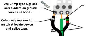
Insulated #6 AWG 600 V solid copper ground wire from locate device to ground rod.
