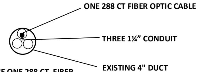
PLACE ONE 288 CT. FIBER OPTIC CABLE INSIDE ONE 1 1/4" CONDUIT
