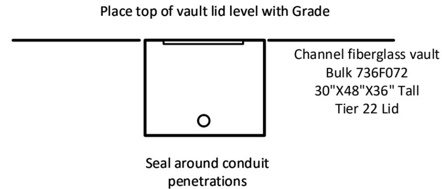
PLACE THREE 1 1/4" HDPE CONTINUOUS CONDUIT INSIDE 4" DUCT.
