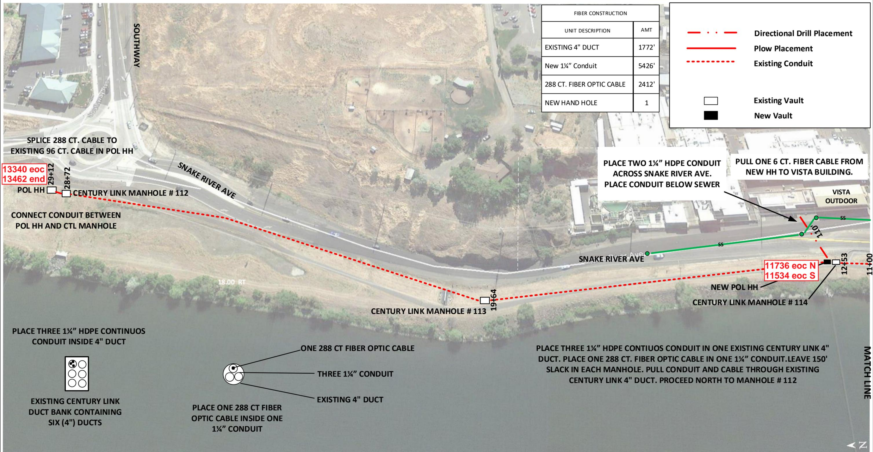
SPLICE 288 CT. CABLE TO EXISTING 96 CT. CABLE IN POL HH
