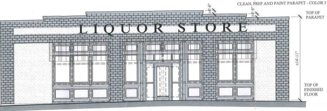
FYPON WINDOW PANELS LOCATED ABOVE AND BELOW SINGLE WINDOW (ON EACH SIDE OF PILASTER) WIDTH WILL BE CUT TO FIT
