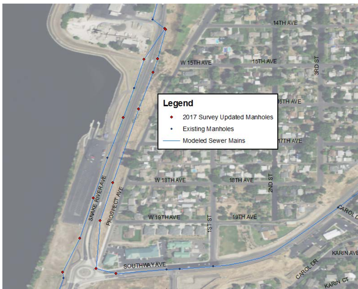
Figure 6 – Southway Ave and Snake River Ave Manholes Surveyed
