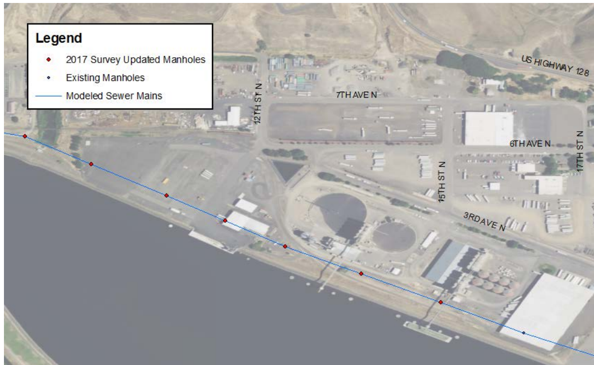
Figure 2 – North Lewiston Manholes Surveyed
