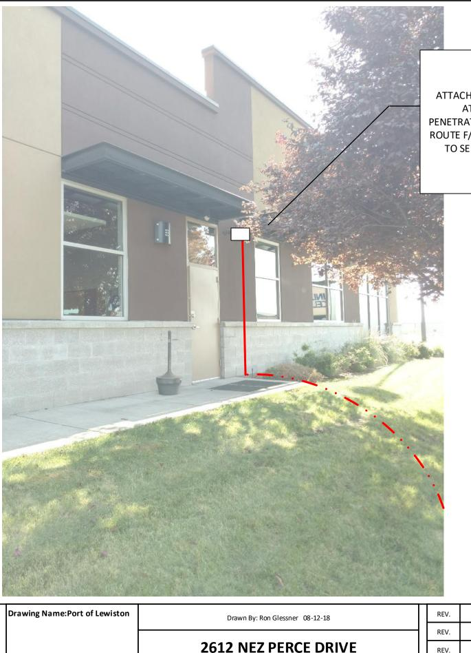
ATTACH 1¼" SCH.40 CONDUIT TO BUILDING ATTACH PULL BOX TO BUILDING PENETRATE WALL ABOVE SUSPENDED CEILING. ROUTE F/O CABLE ABOVE SUSPENDED CEILING TO SERVER ROOM. APPROXIMATELY 50'
