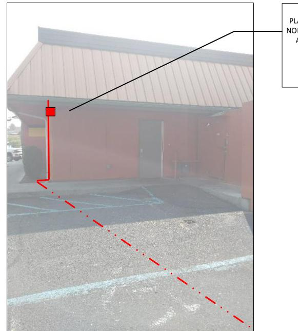
PLACE ONE 1¼" HDPE CONDUIT TO NORTH WEST CORNER OF BUILDING. ATTACH 1½" SCHEDULE 40 PVC CONDUIT AND PULL BOX ON BUILDING. ENTER BUILDING THROUGH ROOF SOFFIT.
