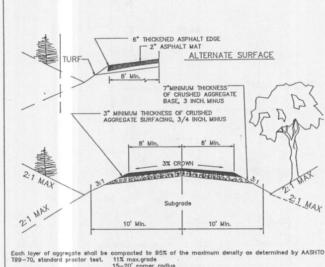
15-20' corner radius 175' centerline radius Swale drainage
